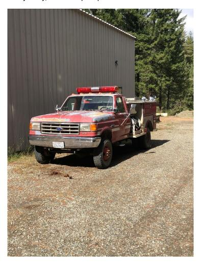
The department's water tender was not at the station, and is routinely stored at a member's home, as it does not fit within the station. The water tender, with a 4,000 gallon tank was received from Hayfork a number of years ago. Staff said that the water tender runs well and is utilized when they have a response to a fire in the community.
